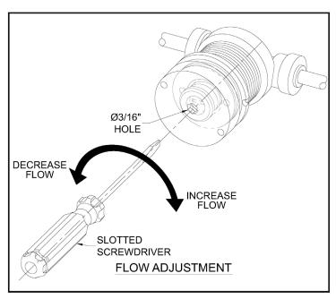
The water flow can be adjusted using a slotted narrow blade screwdriver and turning clockwise to increase flow and counterclockwise to decrease flow.
